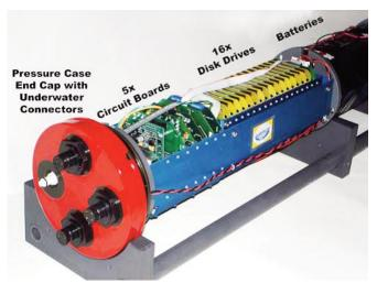
HARP data logger with underwater connectors.
